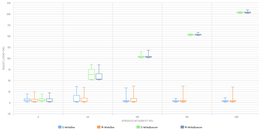
Figure 4.19 – Cassandra write latency using different APIs under manipulated network RTTs among DCs
