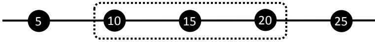
Figure 6.1. A correct replication group for keys in range (5, 10] using consistent hashing with successor-list replication. Replication degree is three and a majority quorum is any set of two in the replication group, i.e., \{10, 15\} , \{10, 20\} , or \{15, 20\} .
