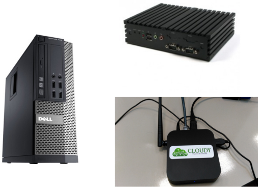
Fig. 3. Hardware used for micro-cloud service provision.
