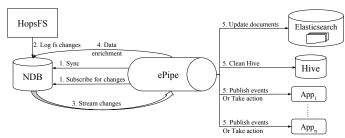
Fig. 1: Architecture diagram of the interactions between ePipe, NDB, and HopsFS. ePipe starts with a recovery phase (sync) to read all unprocessed changes from the database. Also, it subscribes for changes on the logging tables. Whenever a change happens, the database pushes a change event to ePipe, that processes the event(s), and enriches the associated files with extended metadata if available. The enriched events are then published to the subscribers of ePipe.
