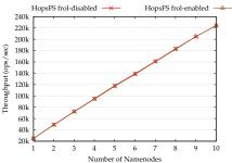
Fig. 3: The overhead of enabling the frol extension in HopsFS for a realworld Spotify workload in which 4.77% of the operations are mutating the namespace (create, delete, rename, and my operations).
