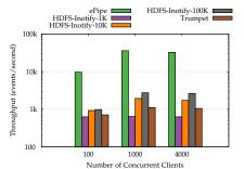
Fig. 5: Comparison of the throughput of ePipe/HopsFS, HDFS INotify, and Trumpet. HDFS INotify clients can set the maximum number of events to request from the namenode, so we compare against three different configurations for HDFS INotify (1K, 10K, and 100K). The default and recommended configuration for HDFS INotify is 1K. The Y-axis is in log scale with base 10.
