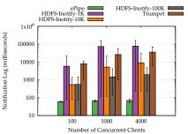
Fig. 6: The average lag time for notification events, that is, the time taken from creating/deleting an inode until it reaches HDFS INotify client, Trumpet client, or ePipe. The Y-axis is in log scale with base 10.
