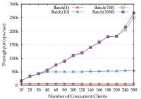
Fig. 10: The effect of batching of AutoIncrement columns in NDB with respect to the number of concurrent clients. The higher the batch size the higher the throughput, however, the auto increment IDs are not serializable across the clients.
