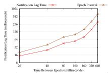
Fig. 7: The average lag time for an event to arrive at ePipe while varying the interval used by NDB to increment the epoch numbers, the default value is 100 milliseconds. The plot is in log-log scale with base 2.
