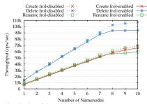
Fig. 4: The overhead of enabling the frol extension in HopsFS. We ran different experiments where 100% of file system operations are logged as Create, Delete, or Rename operations.
