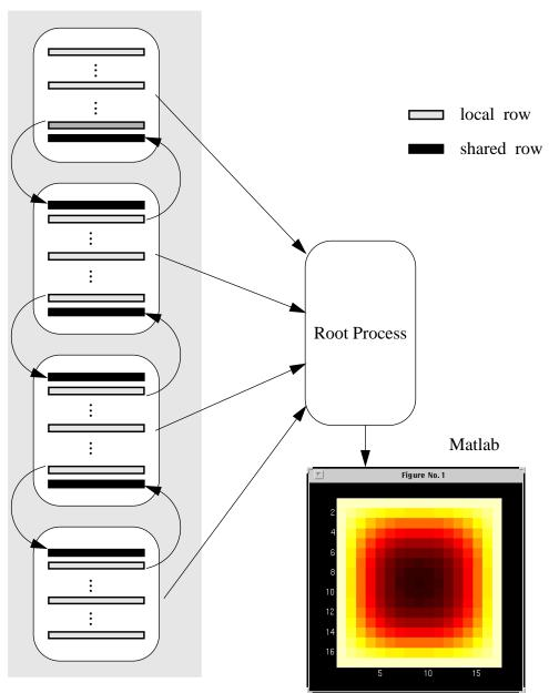
FIGURE 9 Data communication scheme of the Dirichlet problem
